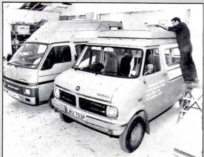
Inside the separate development shop a Bedford CF works van is fitted with a Freschor extractor fan for test purposes. The other vehicle is the second prototype of the Midihome.
