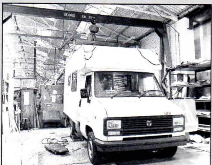
Completed coachbuilt bodies are lowered on to chassis by a 30cwt hoist.
