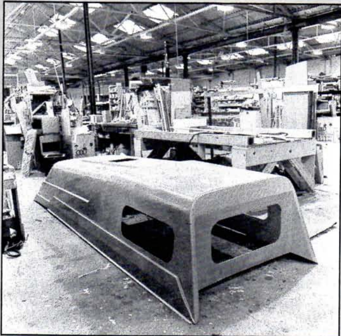
GRP-moulded outer skins for high-top roofs, such as this one for the Midihome, are produced by an outside contractor.
