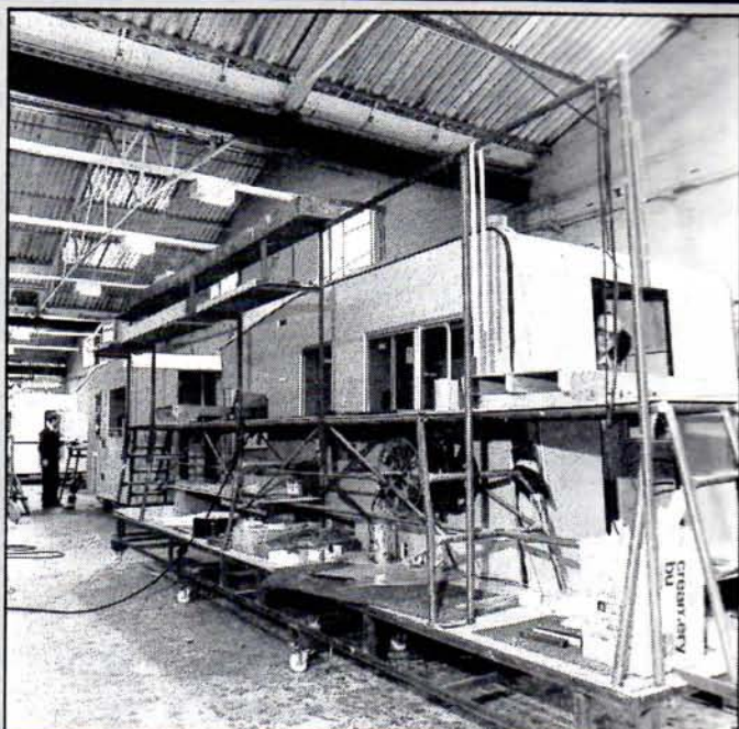
Motorhome and Travelhome coachbuilt bodies were on the main production line during our visit. It's at this stage that the body panels are assembled and furniture is installed.
