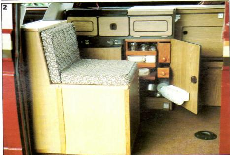
secured by nylon latches, the weight being supported at one side by a plastic shelf support and, on the other, by a hinged leg. A raised edge is fitted to the table for safety reasons.
