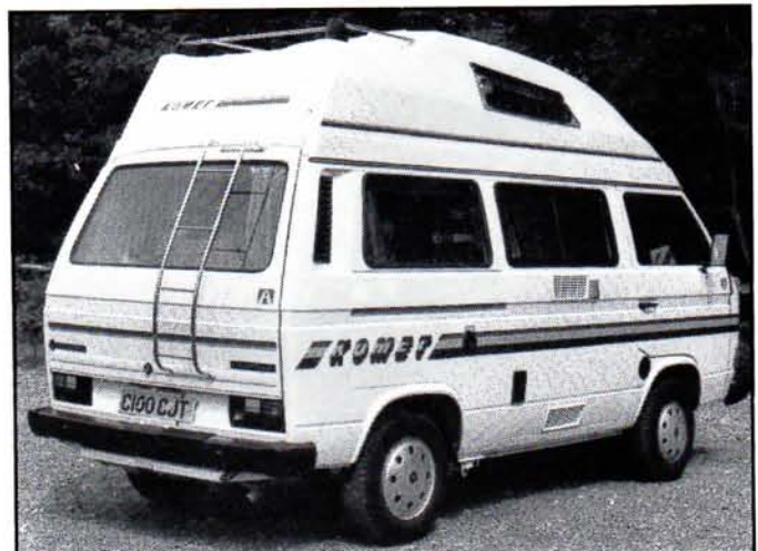
Fixed ladder gives access to rear roof rack
