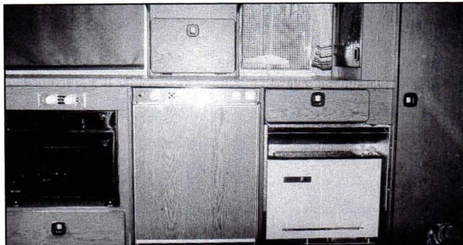
Kitchen unit with oven, 212 fridge, eye level grill and the Carver SD2000.
