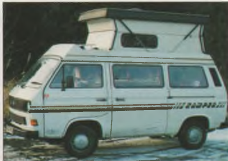
The finished article. Note too the front roof rack, complete with baffle which prevents wind noise.
