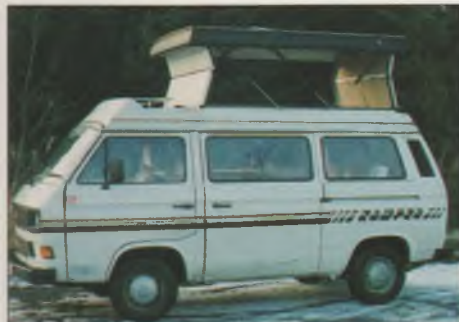
Raising the roof: half-way stage. Gas struts can be clearly seen but side panels are not yet in place.
