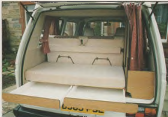
Rear view showing 'parcel shelf', with drawers below. Cushion and drawer unit can be removed for access to engine.
