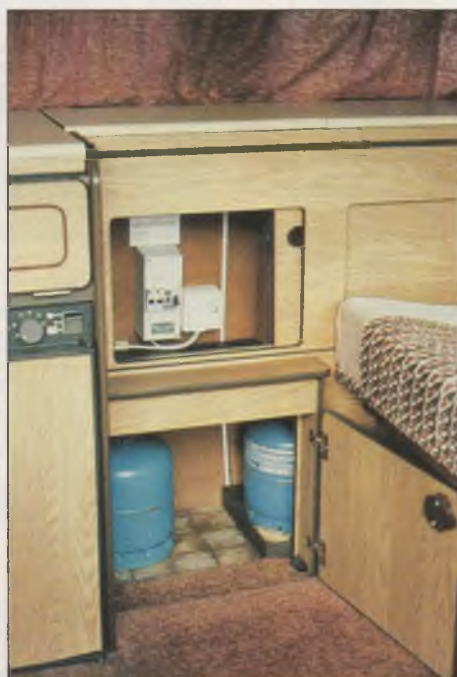
ELCB and refrigerator socket. Storage below for two Camping Gaz bottles, or Porta Potti + one bottle.
