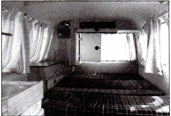
Here is the bed, ready for sleeping bags. There's a locker in the roof above. Wardrobe base (door opened here) projects over bed at rear, so maximum width is at front end.
