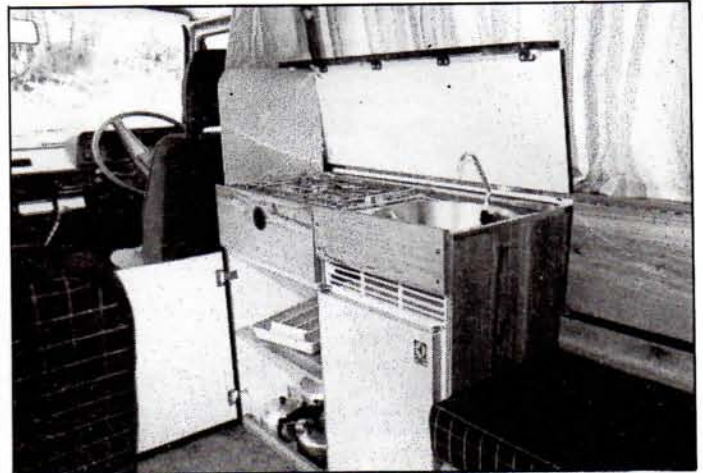
Kitchen unit, behind driver's seat. Opened top provides shelf for pans, splash guard protects front seat. Cooker and sink are integral, all stainless steel.
