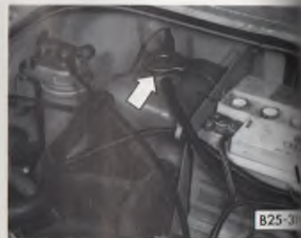
Expansion tank – Diesel engine
