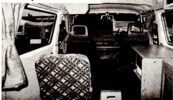
View from rear shows neat cabinetwork with rounded corners. Stool is provided to reach roof.
