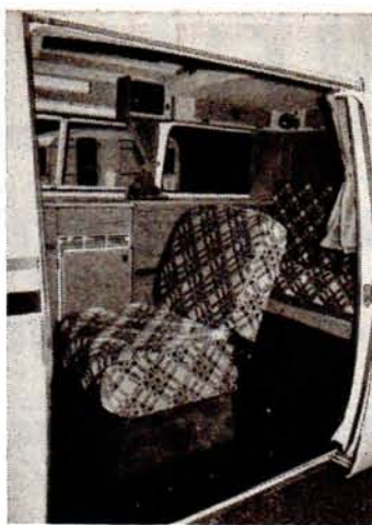
For travelling, rear seat takes two or three, while single seat is turned to face forwards. Note Zig unit over window, small locker and spotlight.
