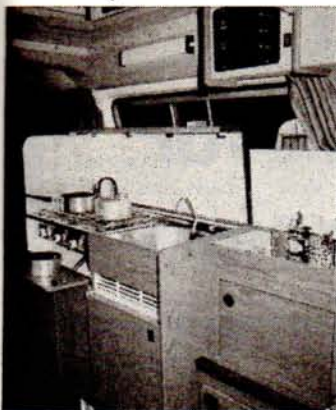
Kitchen arrangement with cooker, sink and separate drainer. Fridge is standard and sliding doors give easy access to upper cupboards.
