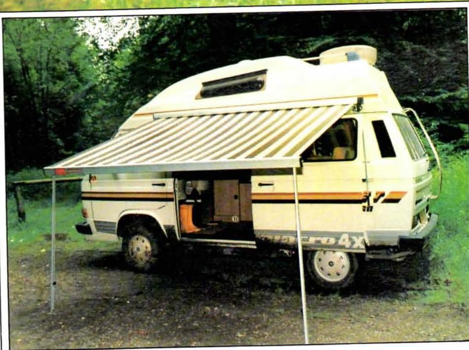
cooker, sink, piped water, storage for a chemical closet and stainless steel roof rack. Like the other Autohomes VW models, body and roof are fully insulated and come with mains electric link-up with earth leakage trip. Among the caravan options are water heater, space heater, TV, fitted crockery, second battery and control panel, waste water tank, child's cab bunk, flyscreen, rear seat restraint belts and the super Fiamma awning which rolls out as a handle is turned. Exterior racks for cycles
